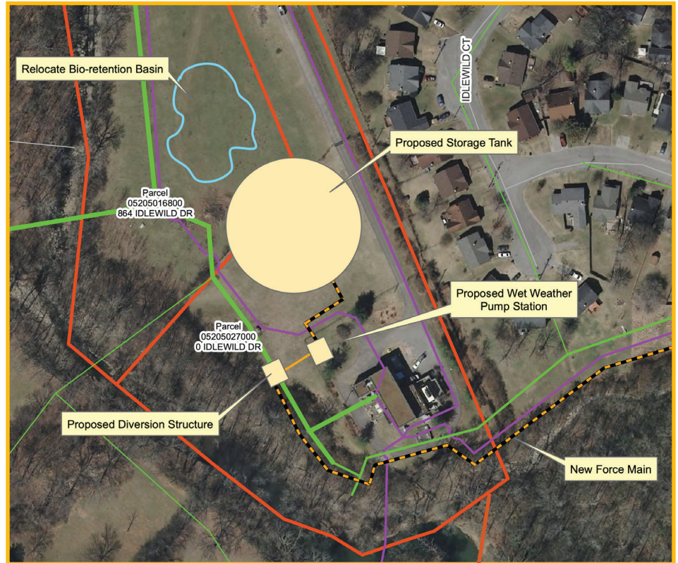
A new storage tank, force main, and new wet weather pump station in the Gibson Creek area are being built to address sanitary sewer overflows.
