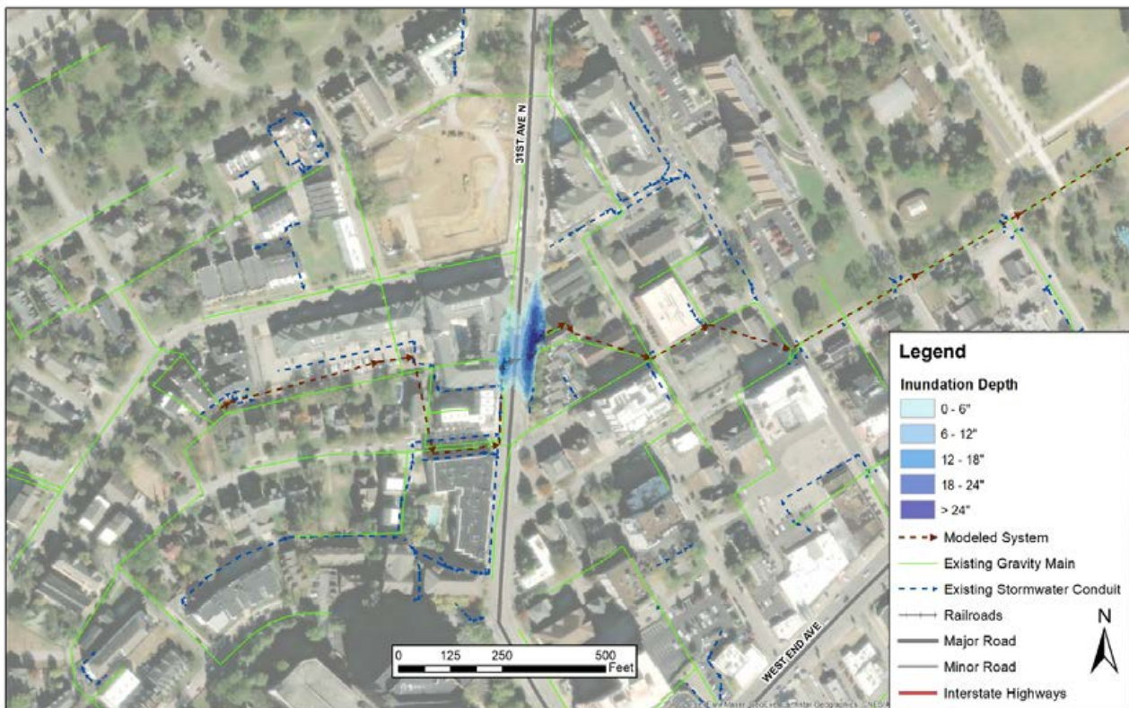
Figure 6-30. Flooding Extents in the 10-Year, 24-Hour Storm, 2045 System
