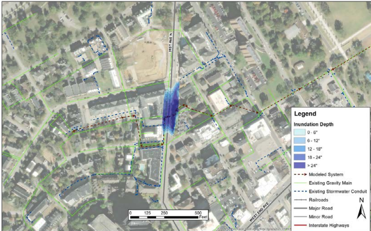
Figure 6-31. Flooding Extents in the 100-Year, 24-Hour Storm, 2045 System
